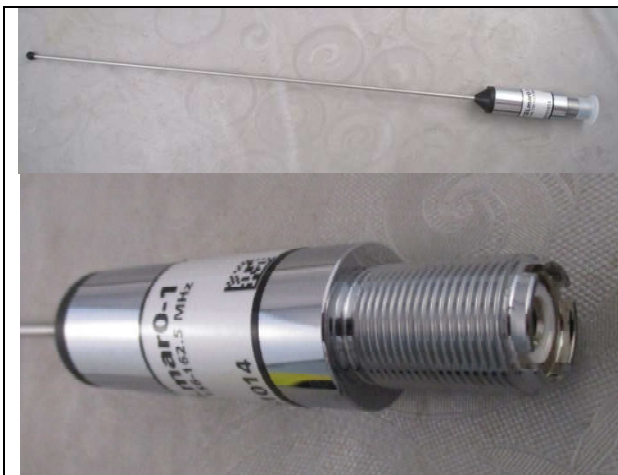
Sample "CELmar" after four cycles salt spray test
