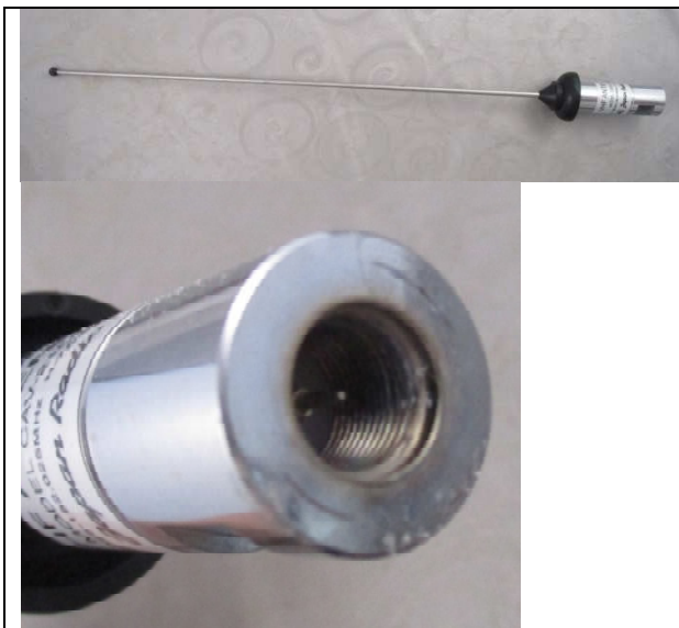
Sample "H7ABJD00027" after four cycles salt spray test
