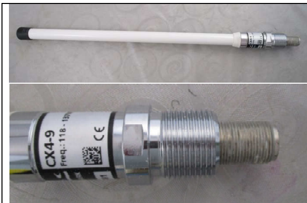
Sample "CX4" after four cycles salt spray test
