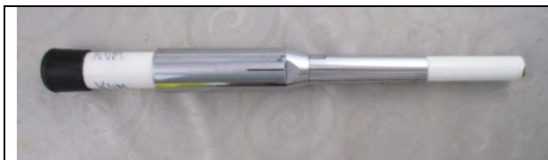
Sample "KUM" after four cycles salt spray test
