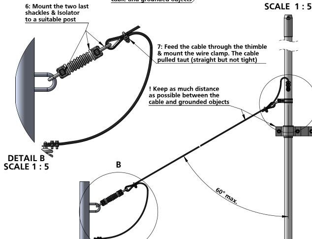
8: Finally the cable clamp must be connected to the antenna tuner max 1m from the wire isolator with a slack cable
