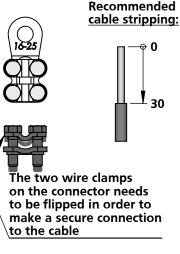
4: Mount the cable clamp pointing upwards to 1: Mount the awoid water ingress in the cable tube clamp and tighten the two 50mm from the nuts by 3Nm antenna screw 2: Mount the shackle & thim and feed the wire through Use wire (not included) to lock the shackle 3: Use anti-sieze on the bolt and fix the nut by 5: Mount the wire clamp max 1Nm leaving slack cable to connect the antenna **DETAIL A**
